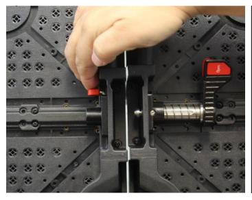
5. Press on the release pin on the receiver latch to release the main shaft of the latch. For side latch the spring latch will automatically spring out of position. For top latch the latch gravity will release the latch
