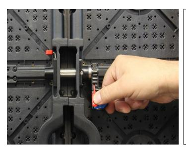
1. Press the red release trigger over the closed latch and hold down wile at the same time turning the latch clockwise to loosen latch
